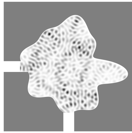
Fig. 2 A contour plot of an electron density in a sample dot for Kd = \sqrt{32}\pi , \tilde{B} = 4 and the fundamental mode incidence.
