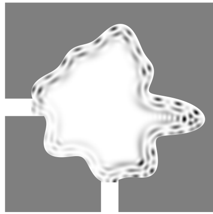
Fig. 6 A contour plot of an electron density in a sample dot for Kd = \sqrt{32\pi} , \tilde{B} = 16 and the fundamental mode incidence.
